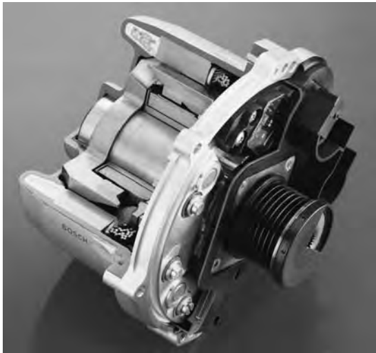
Figure 6.38 Water-cooled alternator (Source: Bosch Press)
